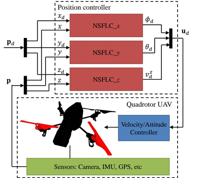
Fig. 2: The NSFLC-based closed-loop control structure for the navigation of the quadrotor UAV.
