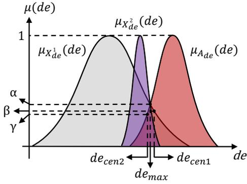
Fig. 4: The difference between the Cen-NSFLC and Sta-NSFLC.  $\alpha$ ,  $\beta$  and  $\gamma$  are the different firing levels.
