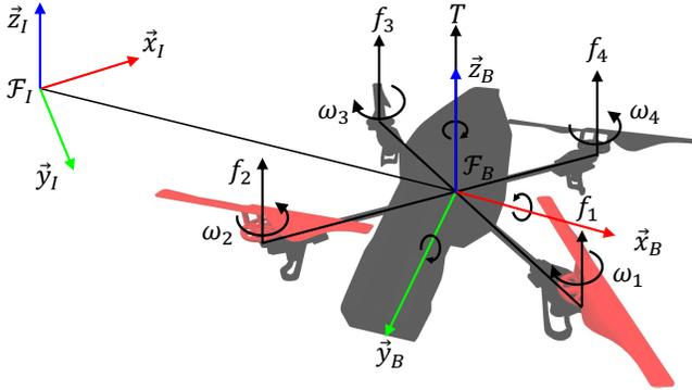
Fig. 1: Quadrotor UAV model with reference frames.
