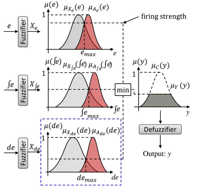
Fig. 3: Example of the calculation from inputs ( $X_*$ ), antecedents ( $A_*$ ) and consequent ( $C$ ) fuzzy sets to output ( $Y$ ) of a Sta-NSFLC.
