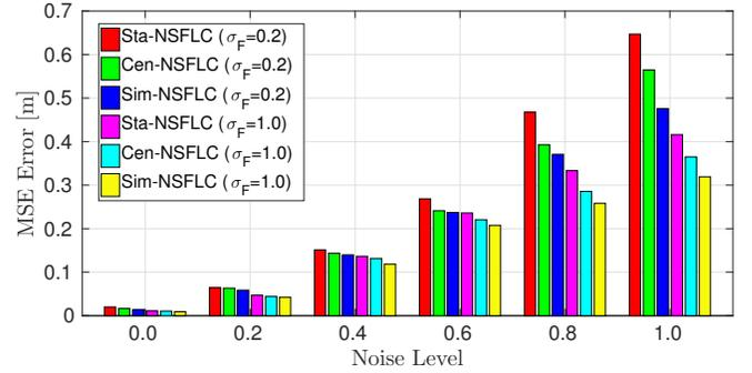
Fig. 7: Control performances of the Sta-NSFLC, Cen-NSFLC and Sim-NSFLC in 3D trajectory tracking task.
