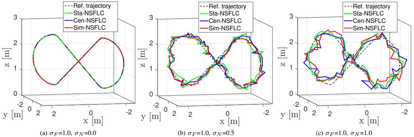
Fig. 6: Example of three UAV flights with the same input fuzzification ( $\sigma_F=1.0$ ) under three different levels of noise.
